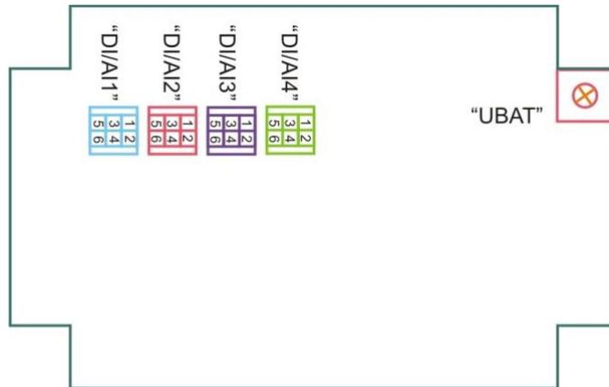
Placing and numbering of configuration pin switches
