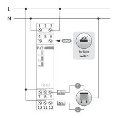
Example application of the PSI-02 transmitter in connection with roller shutter controller: closing of roller blinds at dusk and opening at dawn
