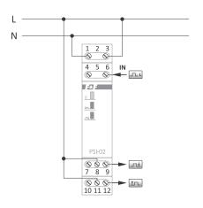
Example of connection with control impulse L
