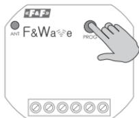
Once the receiver is correctly connected, press and hold the PROG button until the device switches on the output circuit and the communication LED goes out.
