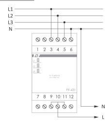
The outputs 9, 10, 11 are connected in parallel, which means that the output signal is available on each of them.
